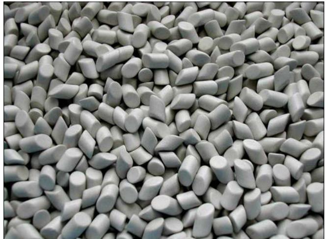
Close-up of the ceramic chips after rinsing and overnight drying ... these measure 4 mm x 5 mm and have their ends cut at an angle to assist with the cleaning and polishing process. This size produced no "jamming-up" inside the cases.
